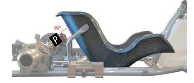
**Height:** Bottom of the seat, level with the bottom of the chassis
