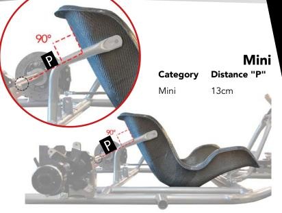
**Height:** Bottom of the seat, level with the bottom of the chassis
