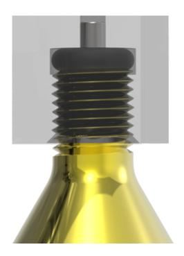
This seal needs to be replaced if you notice a leak near the CO<sup>2</sup> cartridge.
