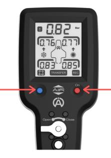
Transfer the pressure as hot tyre pressure
